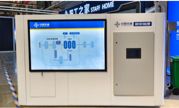
CCCC XI'AN ROAD CONSTRUCTION MACHINERY(XRMC)'s kitchen waste degradation equipment reduced the volume of restaurant waste by more than 95% within 24 hours
