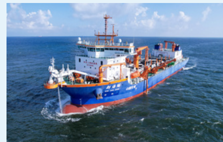
"Xin Hai Xun Vessel" dual-fuel trailing suction hopper dredger
